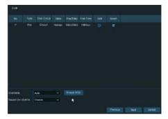
If the HDD is installed in the DVR for the first time, it must be formatted. Select the HDD and then click **Format HDD** button to format the HDD.
